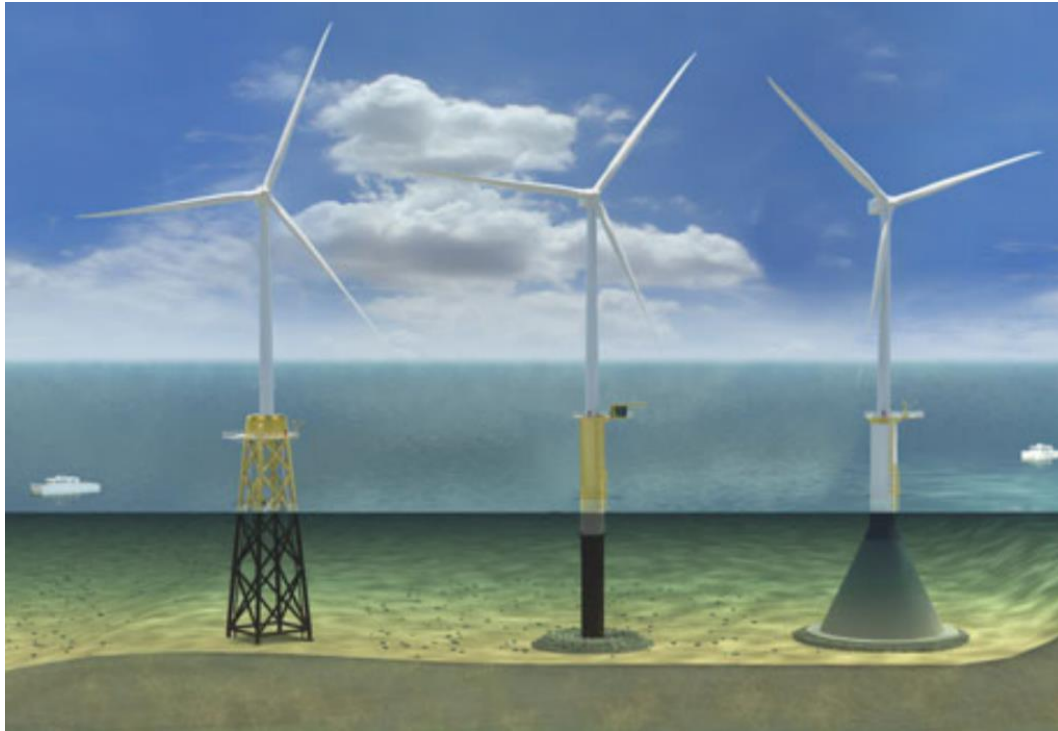
Figure 4.5: Indicative Foundation Options (Multileg, Monopile and Gravity Based Structure) Source: offshorewind.biz
